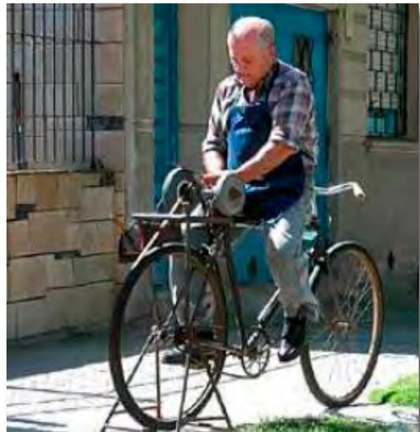
He carried his grinding stone mounted on a rack over the back wheel. When people heard his whistle they came out of their houses and waved. He would stop and pull his bike up onto a stand, then sit on the seat facing backwards, pushing the pedals with his feet. The backward pedaling made the grinding stone spin, and he’d lean over it to sharpen dull blades of all kinds, adding a dash of mineral oil now and then, exchanging news and gossip with housewives and flirting with maids as he worked.
